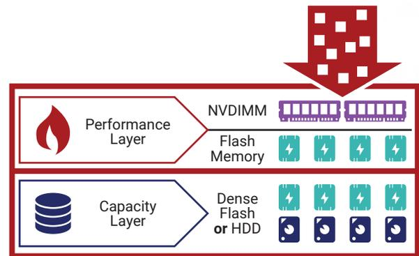
Figure 1. IntelliFlash metadata acceleration and caching architecture
